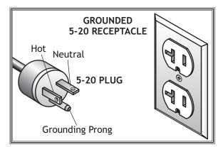
Figure 3. NEMA 5-20 plug & receptacle.
